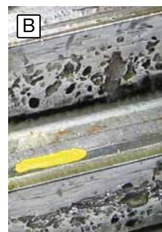
Photo B: Evident smoothing 5 months after changing to Eco Gear 460 M
