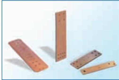
Copper bars, flat and massive, round edges, standard length 4000 to 4200 mm, according to DIN EN 13601 (DIN 46433, DIN 40500-3). Other dimensions on demand. Material of the bars = E-Cu 57 F25 bare<sup>1</sup> (standard), E-Cu F20 and F30 on demand. Mechanical strength about 250 N/mm<sup>2</sup> on E-Cu F25 (standard). Electrical conductivity 56 S x m/mm<sup>2</sup>.
